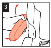
To rotate armrests up or down, pull out on arm and rotate. Make sure armrests lock into place.
